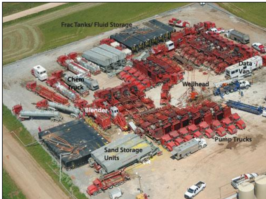
Figure 6: Typical Oil & Gas Hydraulic Fracturing Site Layout
