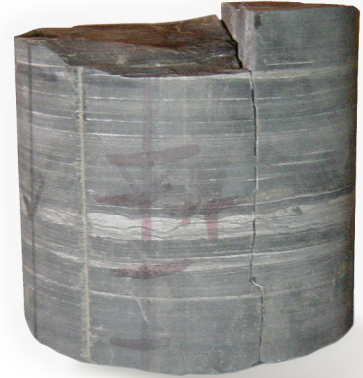
Core from organic Devonian shale formation
