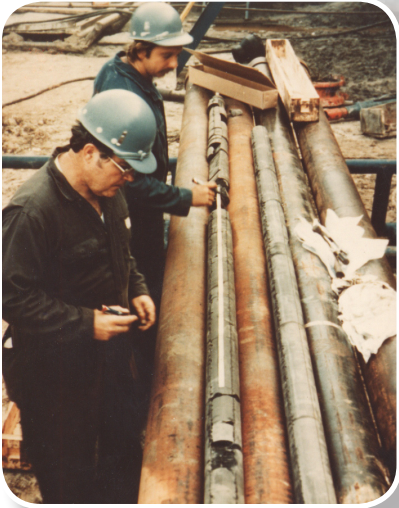
DOE researchers gathering data from one of a series of cored shale wells in the Appalachian Basin in the early 1980s.
